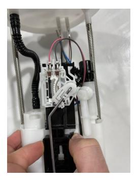
3. Remove the small white retaining clip at the base of one of the support rods. It is easiest to get a small flathead or pick between the clip and the rod and gently pry the clip off. Separate (not completely as there are wires and a tube connecting them still) the top hat from the fuel basket and set the retaining clip and springs to the side.
