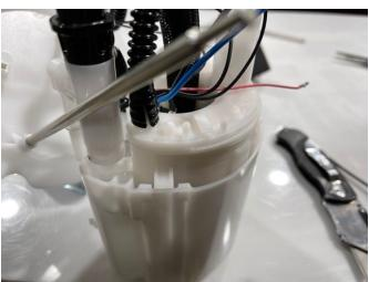
6. Now you can see the two small retaining tabs (top and bottom of the circle in the picture) that keep the pump in its place at the center of the filet and venturi assembly. Using two small screwdrivers or picks, pry those tabs outwards and twist the pump counterclockwise and it should almost fall out the bottom of the assembly.
