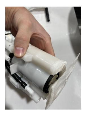
11. Take the included PTFE tube and use a hair dryer or heat gun to slowly and **carefully** heat one end till you can slip it over the barb where we cut and removed the hose from earlier (the fuel filter inlet barb) and secure it with one of the included clamps.
