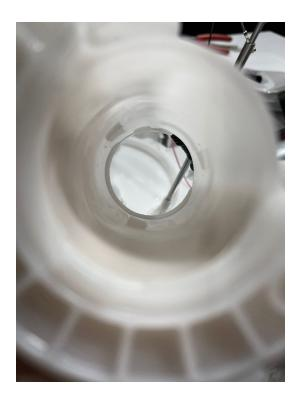
8. If there are large portions of plastic left behind, take a rounded file and remove the leftover plastic as best as you can, being sure **not** to wear through any part of the filter housing.
