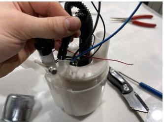
5. You can now squeeze the basket slightly to release the two retaining tabs that keep the pump and filter assembly inside the basket and pull the assembly out.
