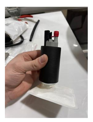
10. Take the fuel pump with the sock and sleeve installed and slide it into the bottom of the filter assembly where the old pump used to sit.
