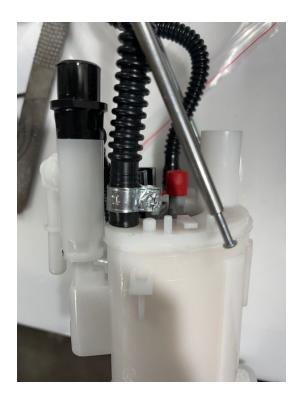
12. Making sure to **be careful** of all of the other plastic parts, slowly heat the other end of the PTFE tube and connect it to the fuel pump outlet and secure it with a clamp. It should look something like this when it is all installed.
