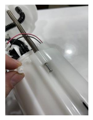
4. Now that you have the top hat removed you can see the pump feed line and the power and ground wires running from the pump to the top hat, disconnect the wires. Take a sharp blade and **carefully** make a small slit in the side of the tube going from the pump to the filter assembly and pull it from the barb as shown below, trying not to mar the white plastic barb underneath.
