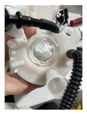
7. Now flip the filet and venturi assembly over and take the same sharp blade from earlier and cit the three small strips of plastic that hold the pump retaining ring to the filter, being careful to not cut into the filter unit.
